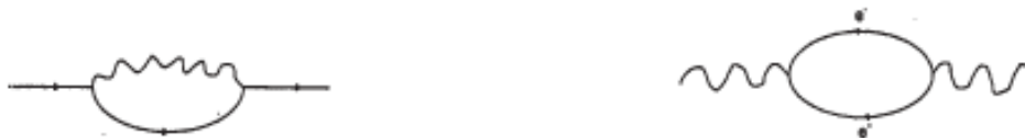
Figure A.1: The Feynman diagrams for electron and photon self-energy. The diagram at left shows an electron which interacts with itself via a photon. The diagram at right shows a photon which spontaneously produces an electron-anti-electron pair which then recombines to give back that photon. These diagrams are primarily meant to be able to write down the terms in the S -matrix expansion, but some physicists tend to attribute a physical reality to them.
